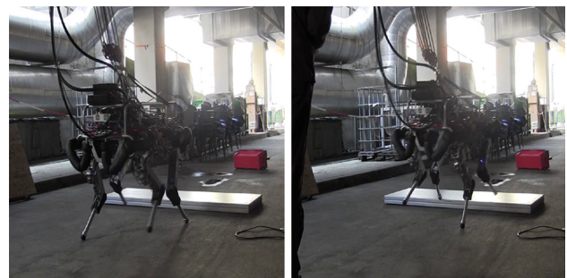
Fig. 13 First outdoor experiment to test the step height modification and heading control while passing over a step of 7.5 cm
